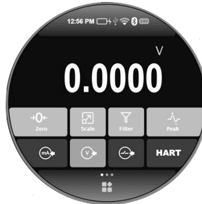
Figure 6 Electrical signal measurement function
